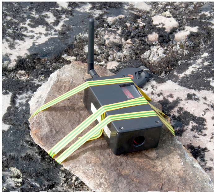
Figure 3.1: A node in the Greenland deployment. The airflow holes and clear window for the light sensor can be seen.
