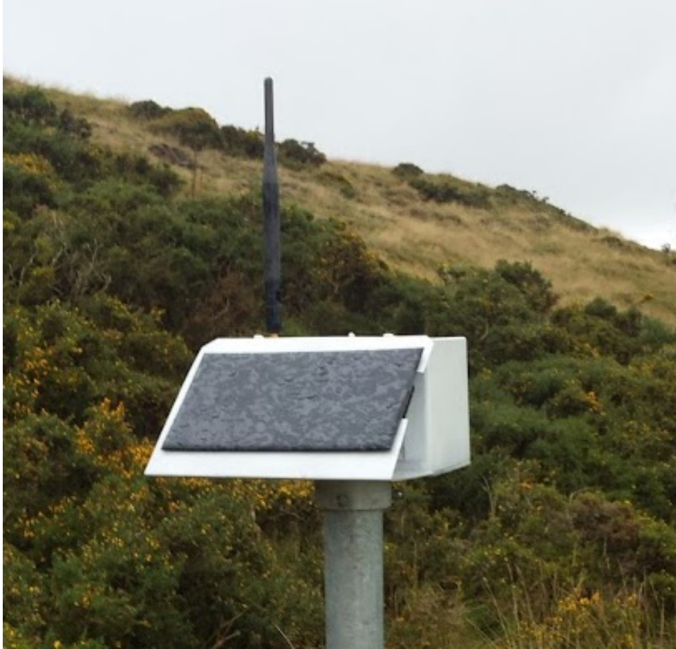
Figure 4.3: Image of a deployed node. The solar panel, antenna, outer case and scaffold mount are visible.
