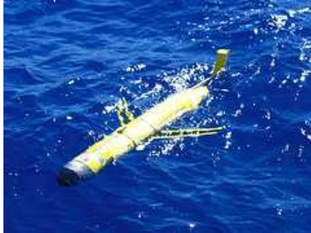
Figure 2.3: The Slocum glider during a test in the Sargasso Sea, the “wings” can be seen in a neutral position keeping the glider surfaced and level. (Image courtesy of Rutgers)
